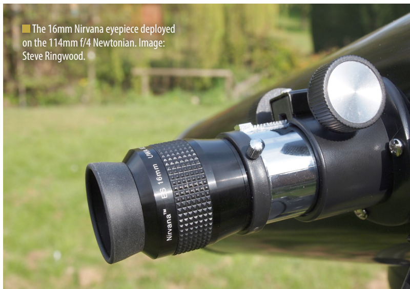
■ The 16mm Nirvana ES eyepiece on the author's 114mm (4.5-inch), f/4 Newtonian. The lightweight eyepieces require no counter-balance measures such as tube shift, even on small instruments. Image: Steve Ringwood.
